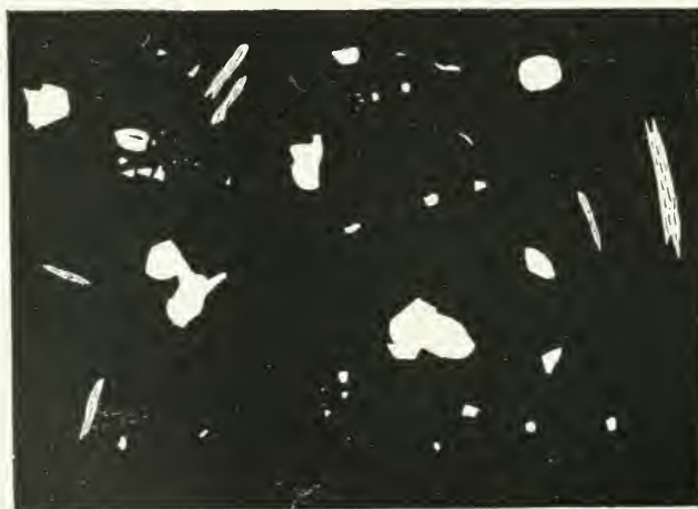
Fig. 37—Character of ore at Garson mine, Sudbury area, Ontario, sixth level. White represents rock fragments, some of which are schists; black represents sulphides. Width of face 5 feet.
